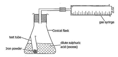
The learner did the experiment three times using different concentrations of sulphuric acid. The same mass of iron powder was used in each case and the experiments were carried out at a temperature of 20°C.
